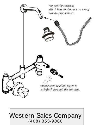
3) In extreme cases, remove the shower riser from the top outlet of the valve, and unscrew the annulus from the top. You can then flush out the valve and pick the rocks out of the annulus. When using the valve as a tub & shower set, you must reinstall the annulus.
