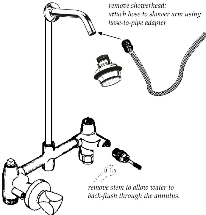
3) In extreme cases, remove the shower riser from the top outlet of the valve, and unscrew the annulus from the top. You can then flush out the valve and pick the rocks out of the annulus. When using the valve as a tub & shower set, you must reinstall the annulus.
