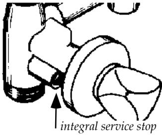
1) **Open the stops.** Yep, slow flow is usually caused by having partially closed integral service stops. The stops are located on the valve body (casting) directly below the stems. The tile-setter might have covered them, but they're there! Open them by turning counter-clockwise with a screwdriver until they touch the copper snap-ring.
