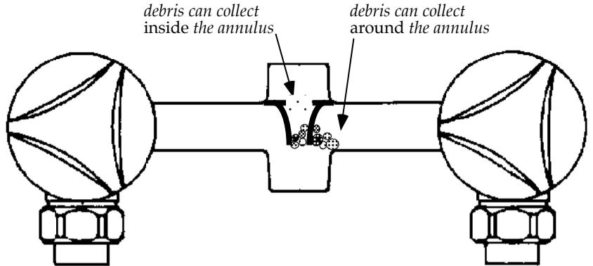
2) The debris can usually be removed by back-flushing the valve through the shower arm with a garden hose. Turn off the stops and remove the stems to allow the junk to flush out of the valve.
